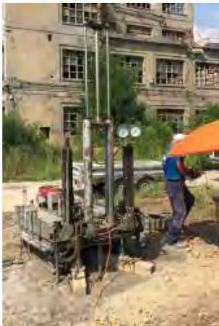
Fig. 4.6 – Penetrometro Deep Drill SP200
